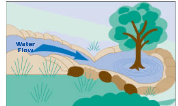
A swale can direct the flow of rainwater to a ponding area that can provide deep watering for trees and shrubs.
