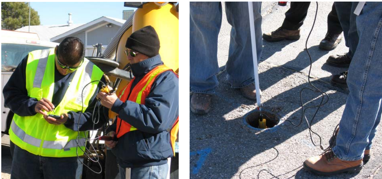
Figure 9: Rio Rancho staff programming data into the PDA and placing a logger on a water valve.
