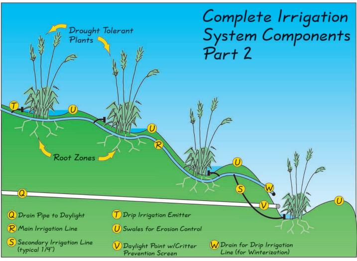
Figure 10-5 (Part 2): The components of a complete drip irrigation system.
