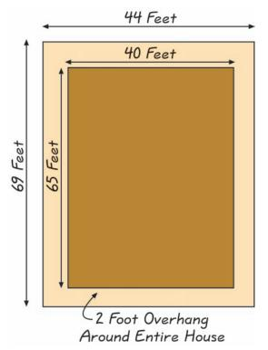
Figure 3-3: Calculating the catchment area including roof overhang
