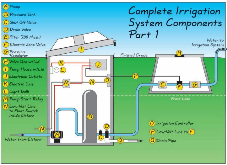
Figure 10-5: The components of a complete drip irrigation system. (Also see next page.)
