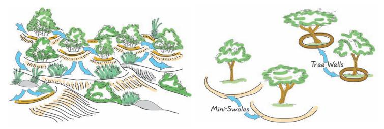
Figure 1-2: Mini-swales or plant pockets (left) are designed to hold some storm water near plants. Tree wells (right) completely circle the root area and can be filled with irrigation water.
