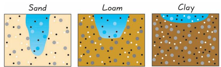
Figure 6-1: Illustration of how soil types affect how water Is dispersed into soil
