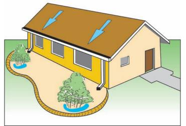
Figure 2-1: A simple ("passive") rainwater harvesting system, with no water storage.
