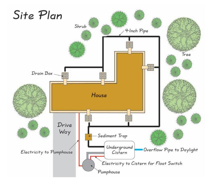
Figure 2-5: An overview of a roof-reliant rainwater harvesting system (water distribution not shown). Conveyance pipes and electrical conduit lines are buried, according to code.
