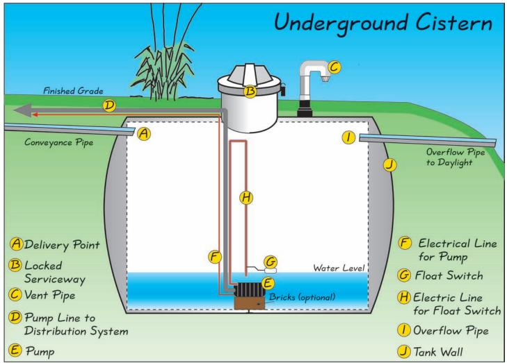
Figure 9-1: This cutaway illustration shows the components of an underground cistern system.
