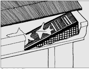
Gutter drain filter.
