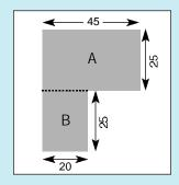
Eva has 1,625 square feet of catchment area. She enters this value in Column C, then multiplies the gallons per SF in Column B by the square footage in Column C to determine the total gallons of rainfall each month. Since the asphalt shingle roof won't shed all of the rainfall, Eva finds the appropriate runoff coefficient (0.9) in Appendix II and enters it in Column E.
